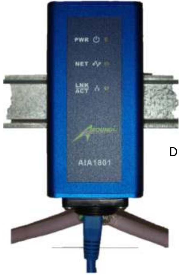
24 VDC Power and Ethernet over same Wire
